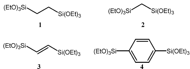
Fig. 1 Structures of the periodic mesoporous organosilica (PMO) precursors. 1 Bis(triethoxysilyl)ethane, 2 bis(triethoxysilyl)methane, 3 bis(triethoxysilyl)ethene, and 4 1,4-bis(triethoxysilyl)benzene
